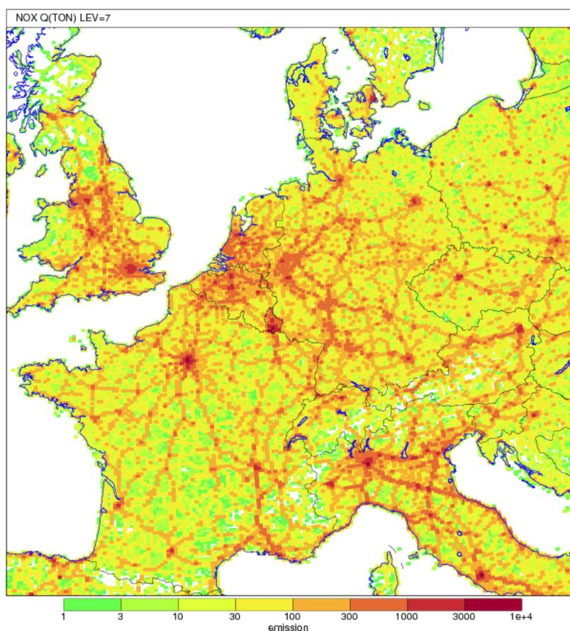
Figure 5: European NO<sub>x</sub> emissions from road traffic during 2009 (approximately 10x10 km<sup>2</sup> spatial resolution).
