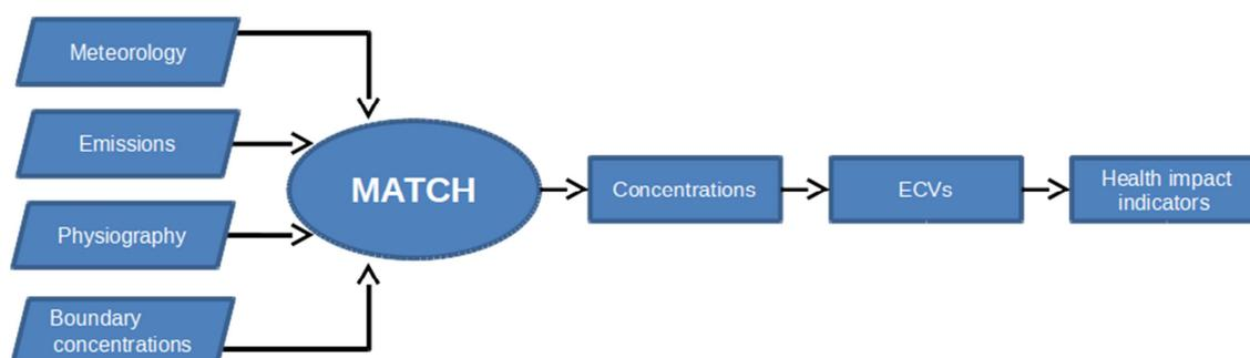
Figure 2 – Schematic structure of the data flow into and out of the off-line model MATCH.
