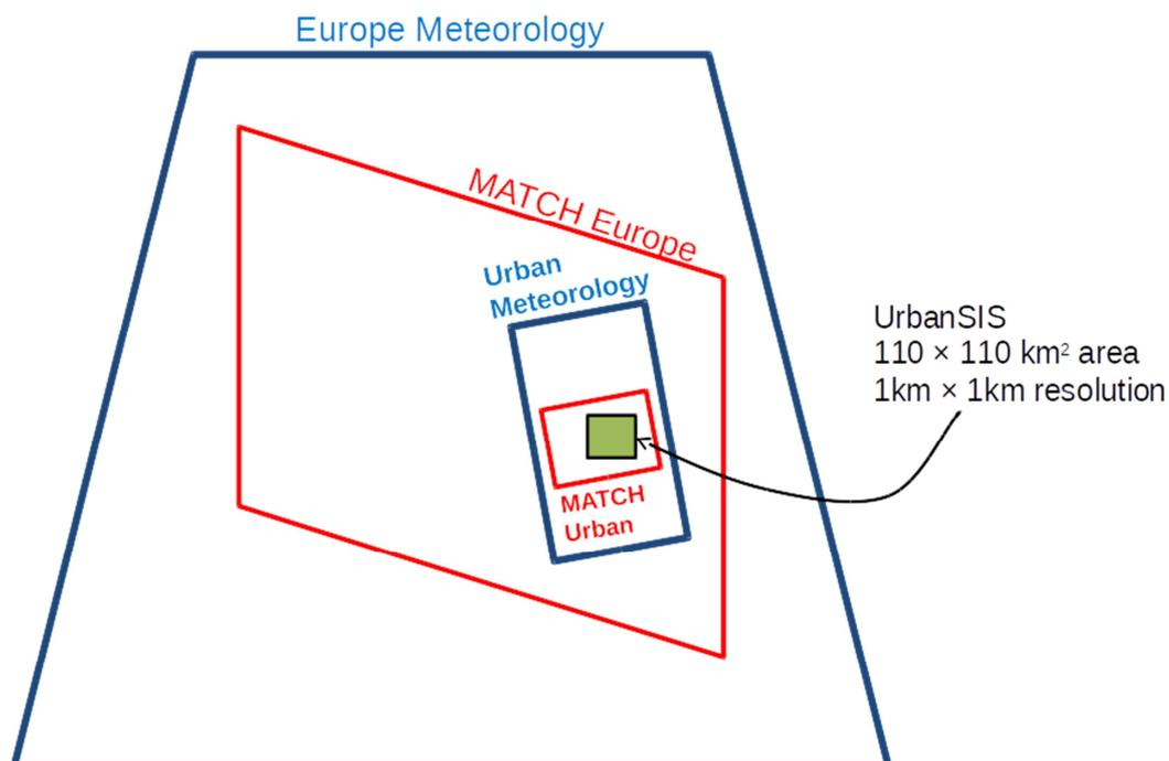
Figure 4 – Nesting of domains in UrbanSIS. The figure is not to scale. The European Meteorological fields produced by HCLIM-ALARO are on a 20 km × 20 km resolution. MATCH-pan-E operates on 0.2° × 0.2° (ca. 22 km × 22 km) resolution, while the urban meteorological (produced by HCLIM-AROME) and air quality applications both run on 1 km × 1 km resolution.
